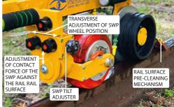
Each search wheel (SWP) is positioned through mechanical adjustments.
