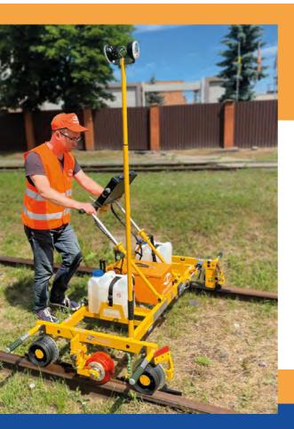
The position of the electronic control and visualization unit (monitor) can be adjusted in three axes. The electronic unit has protection class IP65 according to EN60529.
