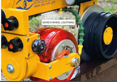
The flaw detector is equipped with special devices that ensure the reliable trajectory of the flaw detector's movement on switches and crosspieces regardless of the direction of movement.
