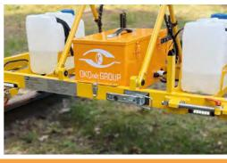
The design includes a system that ensures the search wheel (SWP) is always in the optimal position relative to the rail head during inspection.
