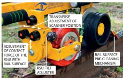
Positioning of each wheel scanner is accomplished by mechanical adjustments.
