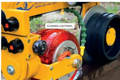
The flaw detector is equipped with special devices that ensure the reliable trajectory of the flaw detector's movement on switches and crosspieces regardless of the direction of movement.
