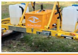
The design includes a system that assures that the wheel (RSUI) is always in the optimal position relative to the rail head during the inspection.
