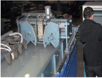
OKO-22M-UT is the best for immersion ultrasonic testing of axles and shafts for the presence of internal discontinuities and changes in attenuation of ultrasonic vibrations in the part material. The system applies all obligatory and additional techniques of acceptance ultrasonic testing, to every testing part, according to international standarts. Specialized Software presents such testing results: amplitude, depth, coordinates and conditional defects sizes.
