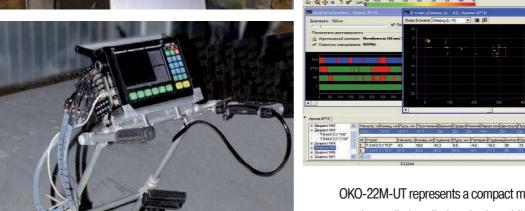
OKO-22M-UT represents a compact module, which can be easily installed on both mobile systems of sheets testing and special industrial cabinets of large-sized automated systems. The number of channels integrated into one system structure can amount up to 200. High performance of pulser and OKO-22M-UT board receiver allows to ensure the generation and receipt of short pulses, with the possibility to minimize the dead zones at the sheet surfaces as much as possible.
