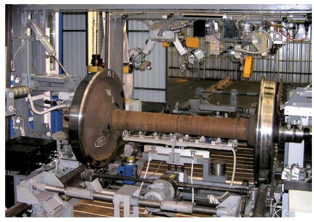
Automated systems for comprehensive non-destructive testing of railway wheel pairs are constructed on the basis of OKO-22M-UT channels. They are intended for automated non-destructive testing of railway wheel pairs by ultrasonic method with the aim to detect such flaws as metal discontinuities, cracks of different orientations, surface defects.
