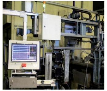
The on-line weld profile monitoring system provides the internal and external profiles of the tested weld and HAZ area along with its thickness. The material thickness and profile alarms notify the operator when the product does not meet calibration parameters. Extremely hard environment conditions are applied by IP64 OKO-22M-UT blocks. Fast Software provides high-speed tube testing with 10 channels simultaneously.
