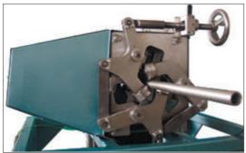
High-frequency measurement provided by Eddycon D flaw detector allows to design high-speed rotary systems for pipes and bars testing, using the rotary ECPs for detection of unacceptable surface flaws.
