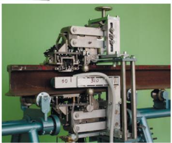
Building of automated eddy-current system for rails testing equipped with Eddycon D multichannel flaw detectors into a production line allows to avoid the necessity of "balancing" on each rail to be tested, due to the possibility of saving the balancing parameters on the calibration block.
