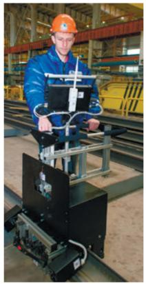
Testing of linearly extended objects with simple or complicated configuration for the presence of surface flaws.
