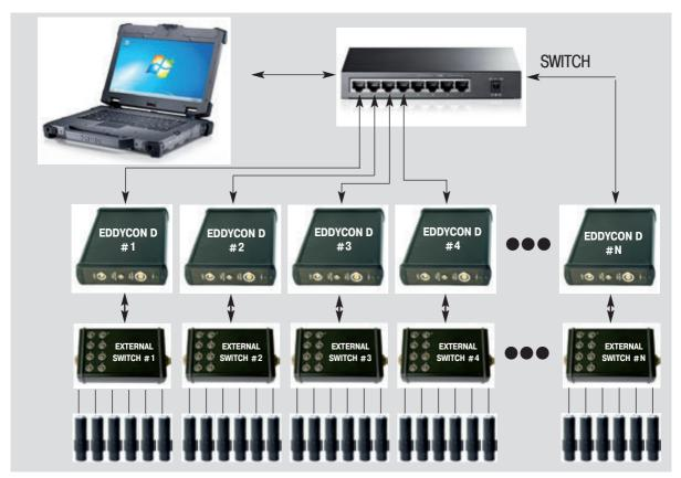
Figure 1. Scheme for constructing the multi-channel system
