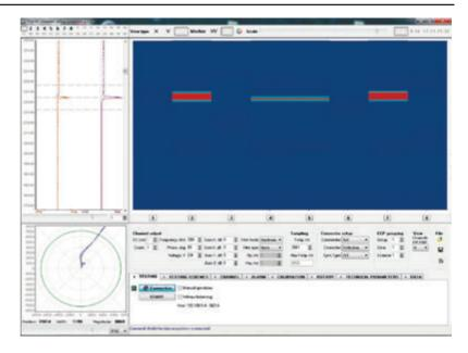
Interface example of a program for setting-up the EC channel
