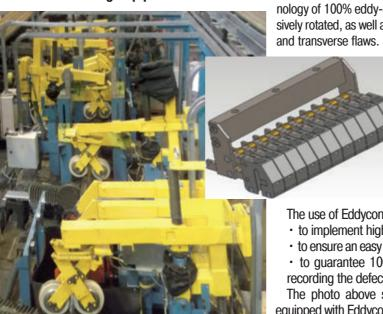
Construction of multichannel systems for implementing the technology of 100% eddy-current testing of pipe body when progressively rotated, as well as for simultaneous detection of longitudinal and transverse flaws
