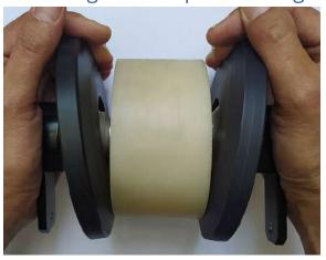
Position of the scanning units on the rail head surface has a transverse adjustment. The transverse adjustment ensures the setting of the scanning units for successful ultrasonic testing of rails of any dimension and wear rate (permissible by the standards).
