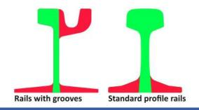
The rail flaw detector deploys a unique scanning scheme that allows you to test the entire section of the rail, except for the foot flanges and the checkrail, using the pulse echo, echo-shadow and echo-image methods.
