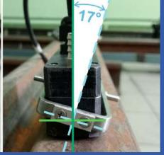
(independent) suspension system and transverse angular degrees of freedom ensuring constant acoustic coupling when the flaw detector deviates from the rail vertically within 17 degrees both to the left and to the right.
