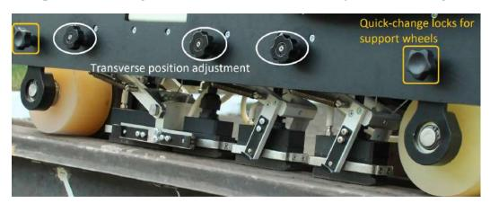
Each probe unit has its own (independent) contact liquid system with a check valve for liquid. For quick and easy couplant refilling, the tank can be unbolted and installed without liquid loss thanks to a quick-release valve with automatic safety lock. The average liquid consumption is 1 liter per 1 kilometer (0.42 gal per mile) of testing.
