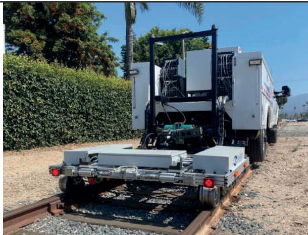
b) equipment installed in the vehicle body (UT channels, automation and control box, hydraulic station, air compressor, container for coupling liquid, water supply system, hydraulic system for lifting and lowering the trolley).
