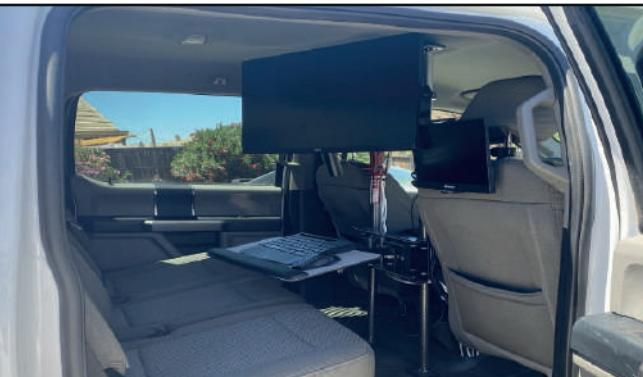
c) the operator's workplace with control monitors is located at the rear seat in the vehicle cabin.
